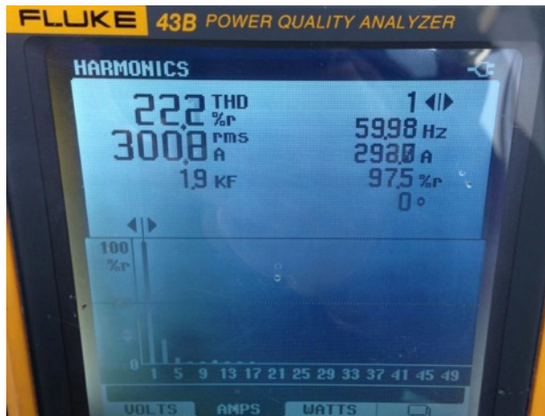
Figure 7: The FFT of the high phase leg shows that it carried 300A of current, 63.8A of which was 3 rd harmonic and 16.8A of which was 5 th harmonic.
