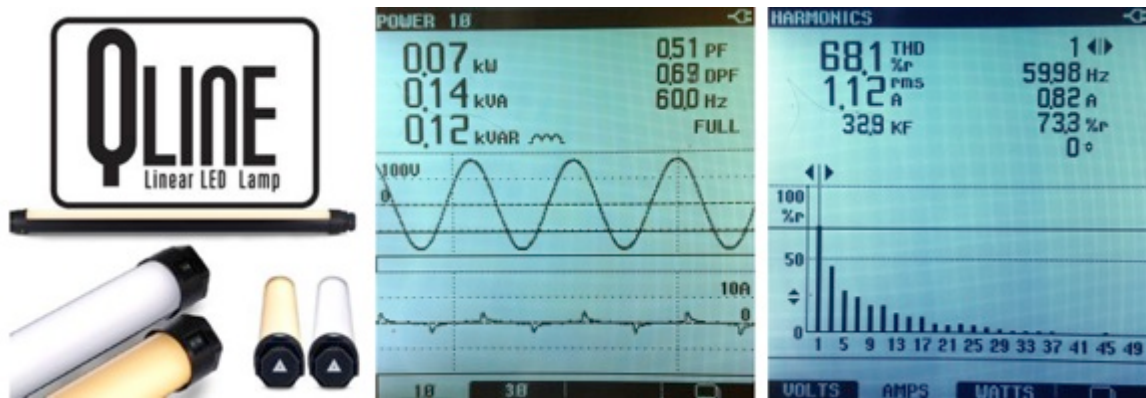
Figure 6: PQM readings of the Quasar Science LED tubes. Note: disproportionate amount of 3 rd order harmonics (3 rd , 9 th , etc.) in the FFT on the right)
