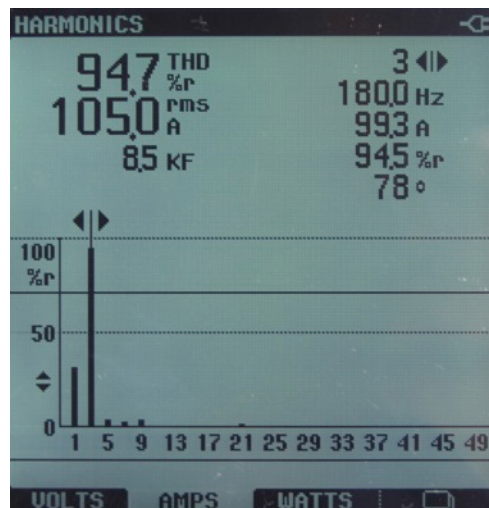
Figure 8: Of the 105A returning on the neutral 99.3A consists of 3 rd harmonic current.
