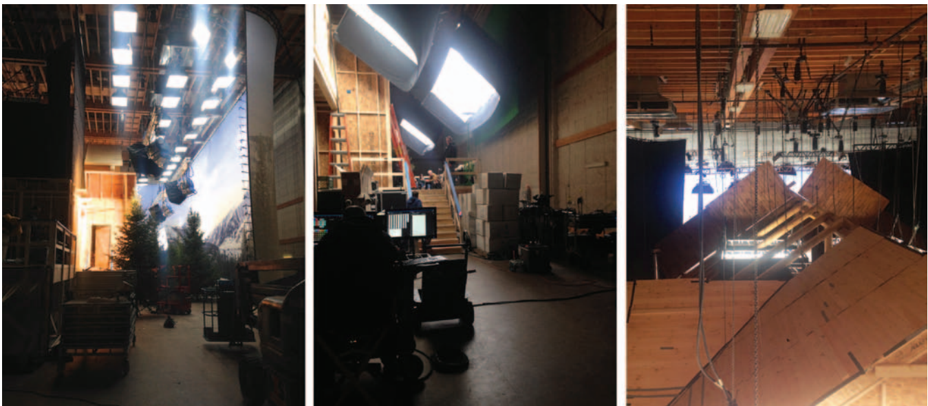
Figure 9 – (Left) 24 kW tungsten fresnels create the feel of direct sun. (Middle) Large soft boxes consisting of 8' Quasar Science LED tubes creates the feel of sky shine. (Right) Smaller soft boxes consisting of 8' Quasar Science LED tubes creates ambient light in the interiors of the set.
